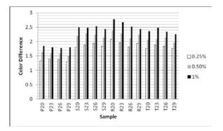
FIGURE 5. Color difference of samples after dyeing in weft direction.
