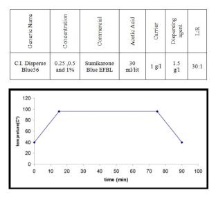
FIGURE 2. Time-temperature curve of sample dyeing.
